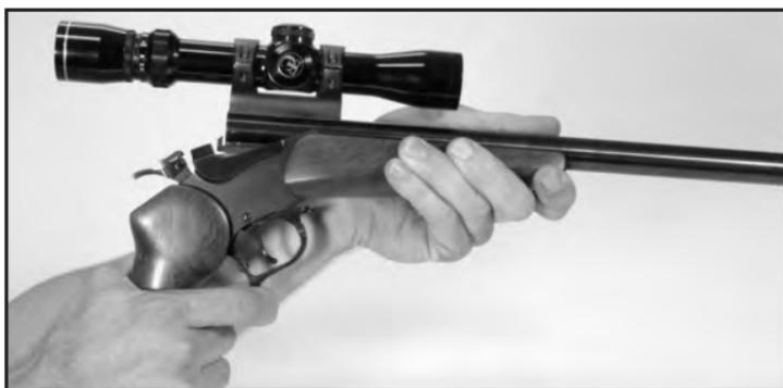
The G2 Contender is a single shot, break-open style firearm. To open the G2 Contender, hold the gun with your left hand at the balance point on the forend. (Use right hand if you are left handed). With your other hand, pull rearward and upward on the trigger guard spur with your trigger finger. Place your finger low on the spur for maximum leverage, and give it a fast, sharp pull. Pull rearward and up at the same time.
