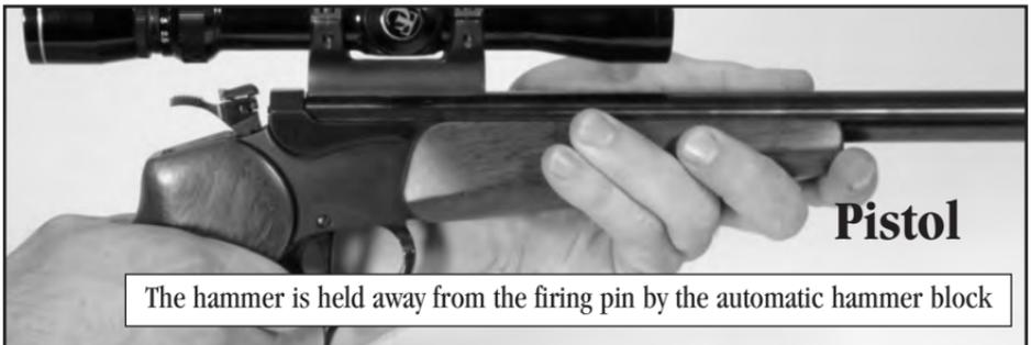
5. Open the action - remove the cartridge.
