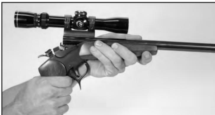
Pulling back on the trigger guard spur will allow the barrel to pivot downward. To close the G2 Contender, pull the barrel upward while securely holding the grip of the G2 Contender stationary with your right hand. Practice
